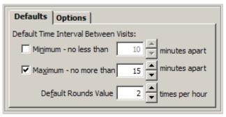
You can select values for the **Minimum** and **Maximum Time Interval** between visits to a location. These values apply to all views except Rounds view. If the time between location reads is less than the minimum or greater than the maximum, an exception is noted on the worksheet.
